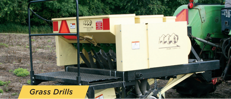
Photo of no-till seed drilling. Seeding natives with a Truax FLXII grass and grain drill. No tillage is necessary prior to seeding because this drill is designed to plant the seed into existing sod.
